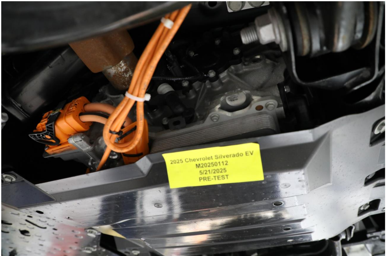
No. 305-23 Pre-Impact Close-Up View of High Voltage Leads Attached
