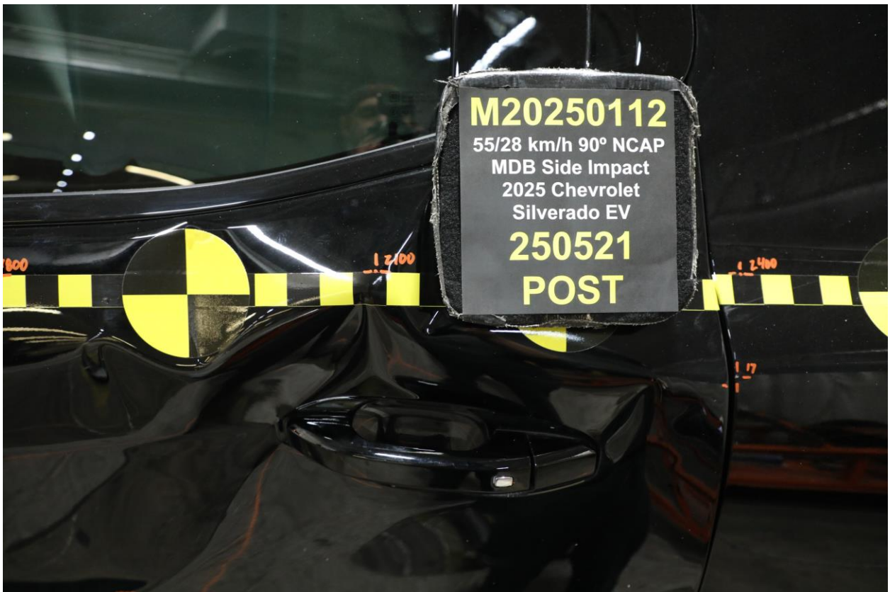
024 Post-Test Left Rear Door Latch Close-Up
