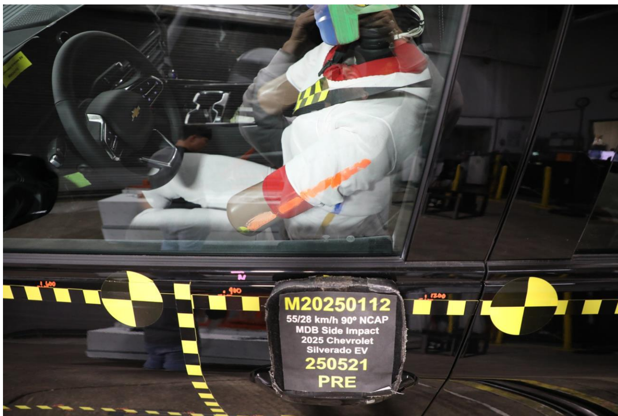
042 Pre-Test Driver Dummy and Door Clearance View
