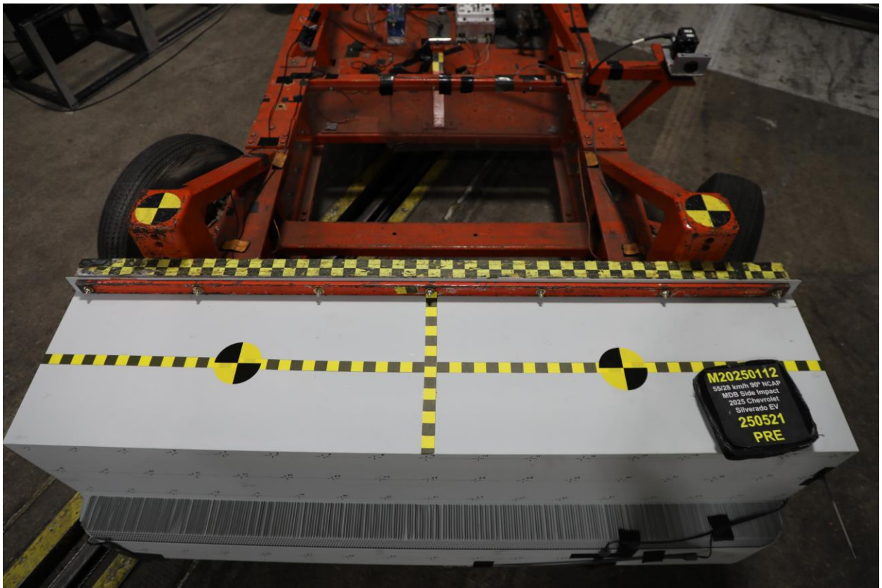
086 Pre-Test Top View of MDB Impactor Face
