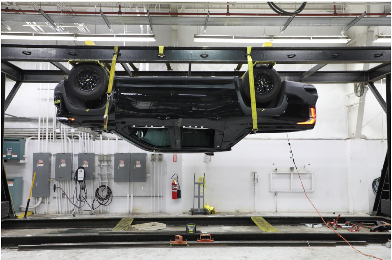
No. 305-29 FMVSS No. 305 Static Rollover at 180°
