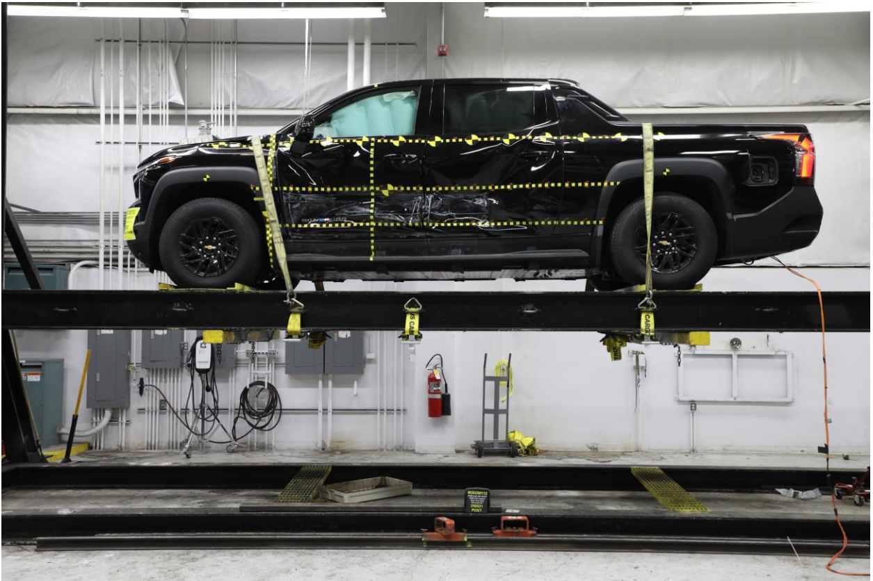
096 FMVSS No. 301 Static Rollover 0 Degrees
