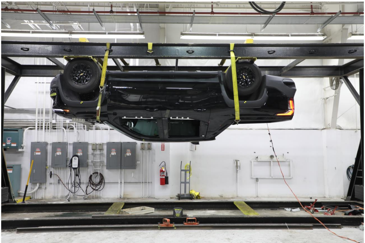
098 FMVSS No. 301 Static Rollover 180 Degrees
