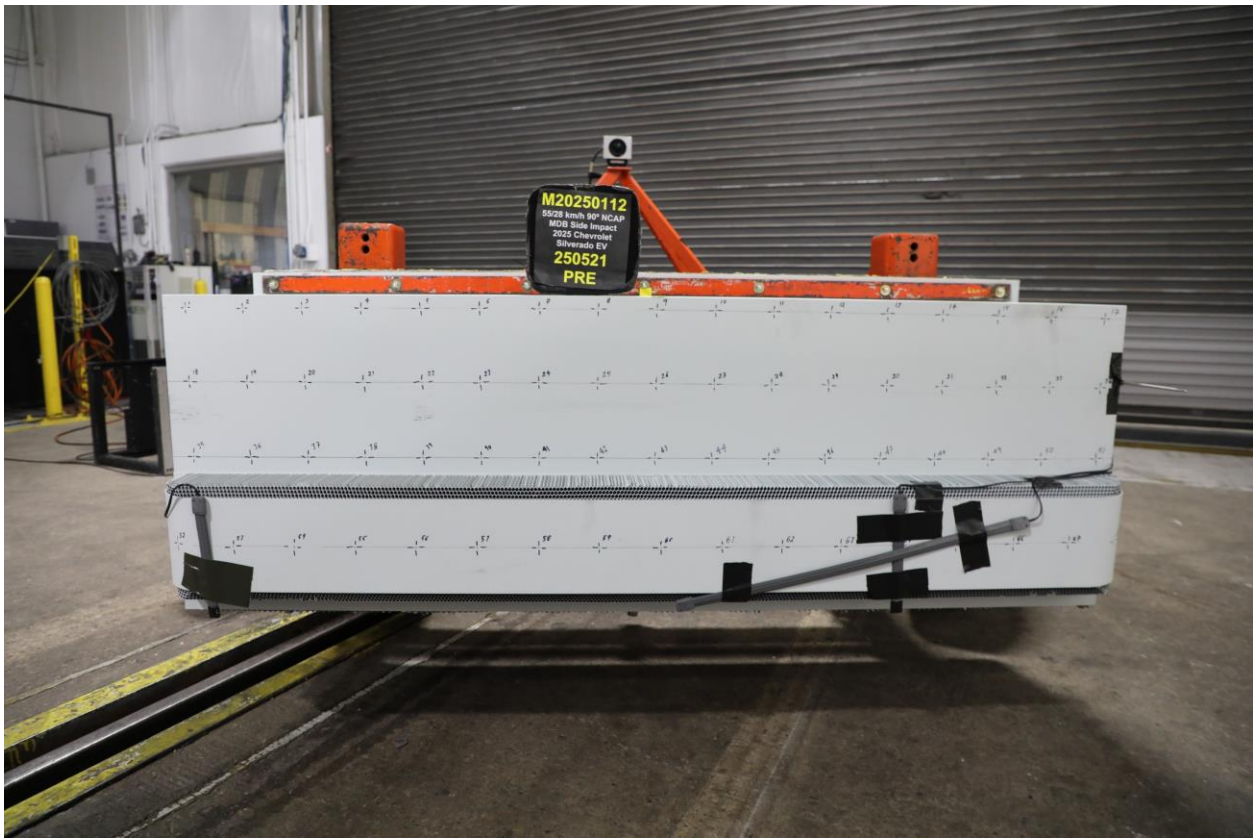
084 Pre-Test Front View of MDB Impactor Face
