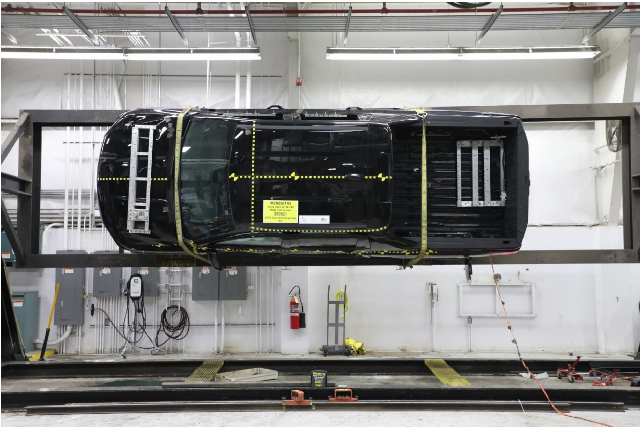
097 FMVSS No. 301 Static Rollover 90 Degrees
