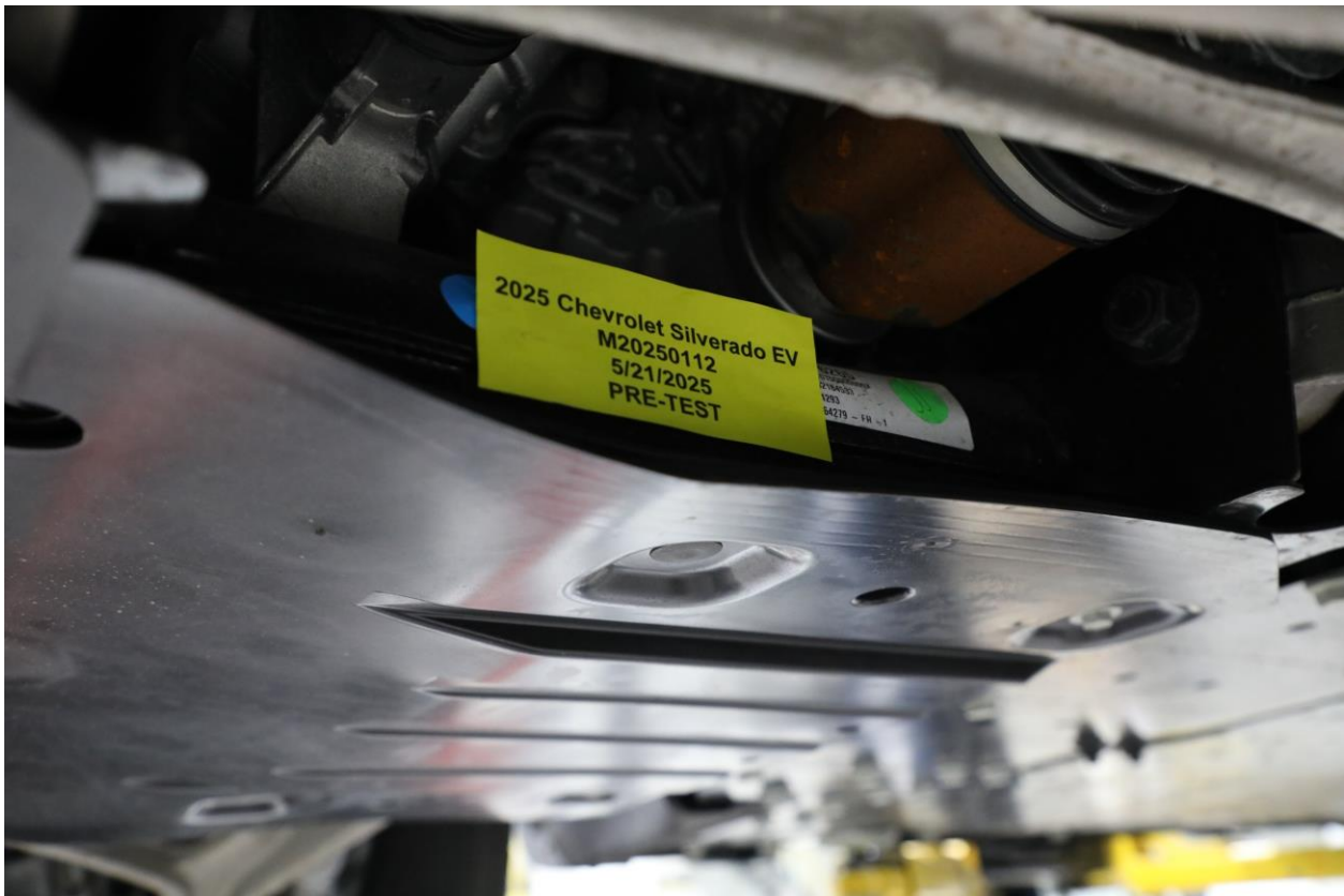
No. 305-12 Pre-Impact View of Battery Box(s) or Container(s) Which Holds Individual Battery Modules
