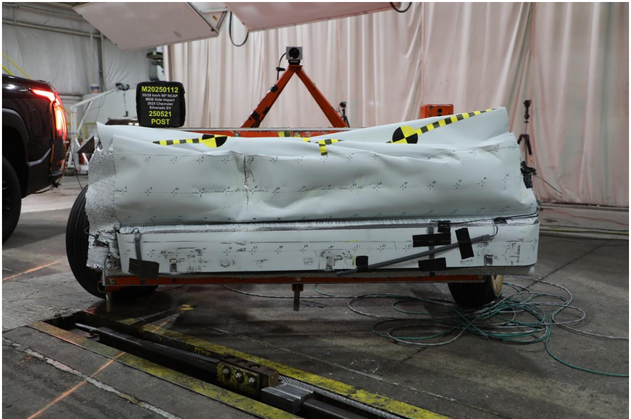
085 Post-Test Front View of MDB Impactor Face
