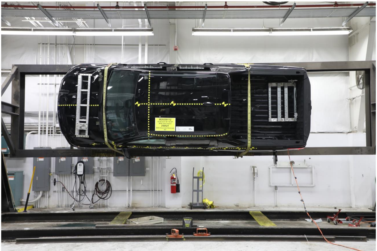
No. 305-28 FMVSS No. 305 Static Rollover at 90°
