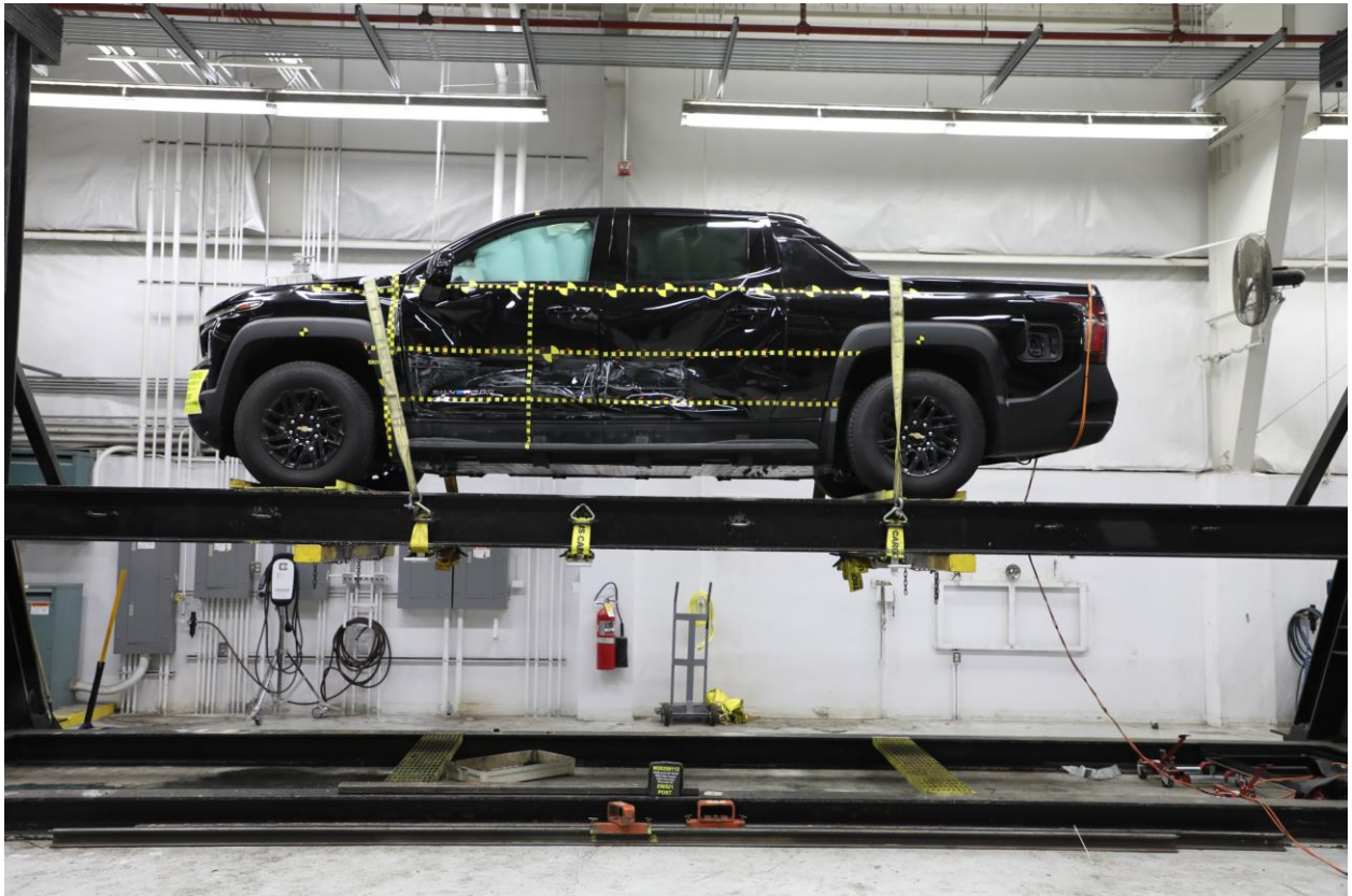
No. 305-31 FMVSS No. 305 Static Rollover at 360°
